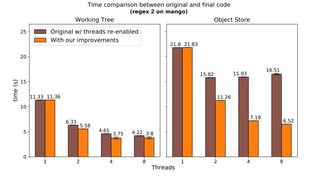
**Figure 7.4:** Time comparison between the original git-grep code and the final code with the patches from this project. Tests executed with regex 2 ("(static|extern) (int|double)  $\times$ ") on machine mango (see Appendix A).
