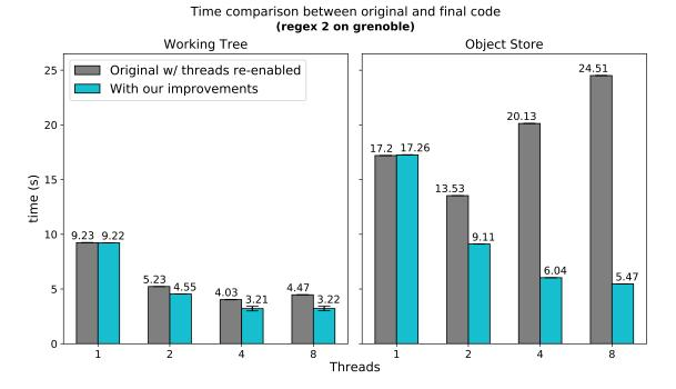
**Figure 7.2:** Time comparison between the original git-grep code and the final code with the patches from this project. Tests executed with regex 2 ("(static|extern) (int|double)  $\times$ ") on machine grenoble (see Appendix A).
