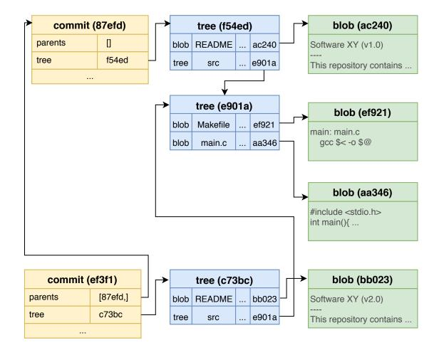
Figure 4.2: Example diagram of Git objects being reused.
