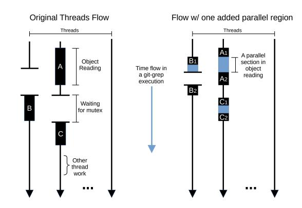
**Figure 6.1:** Diagrams representing the git-grep threads flow. The left side corresponds to the original code. The right side corresponds to a modification adding one parallel region inside object reading. Note how, in the right,  $B_1$  might execute between  $A_1$  and  $A_2$ , possibly changing global variables and breaking invariants that were previously ensured in the original code.
