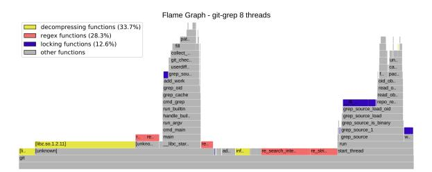
**Figure 5.4:** *Vizualization of* perf's profile for cached git-grep in chromium's repository with 8 threads.
