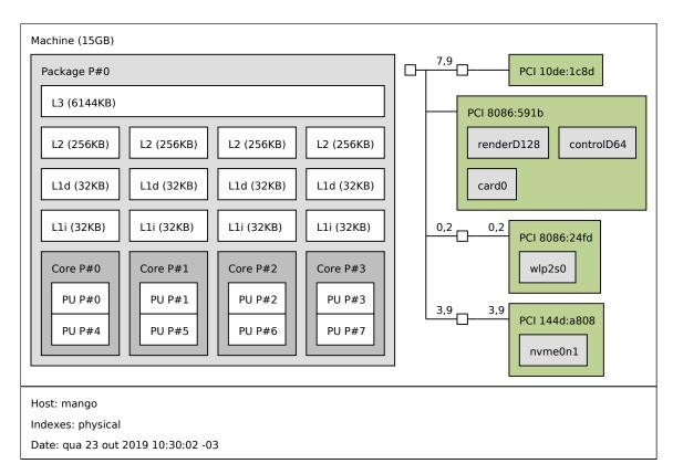
**Figure A.1:** Topology of the machine mango. (Generated with lstopo from the hwlock package.)
