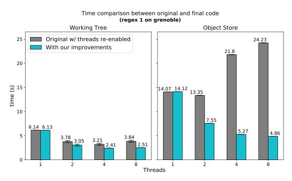
**Figure 7.1:** *Time comparison between the original git-grep code and the final code with the patches from this project. Tests executed with regex 1 ("abcd[02]") on machine grenoble (see Appendix A).*
