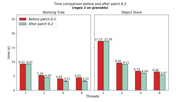
**Figure 7.6:** Time comparison of git-grep's code before and after Patch 6.2. Note that the "before" version already has parallel access to decompression. Tests executed with regex 2 ("(static|extern) (int|double) \\*'") on machine grenoble (see Appendix A).
