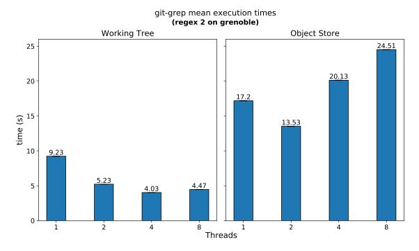
**Figure 1.2:** Mean elapsed time of 30 git grep executions in chromium's repository with regex 2 ("(static|extern) (int|double)  $\times$ "), for different parameters. Executed on machine grenoble (see Appendix A).
